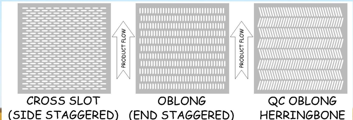
With the QC Herringbone pattern, it is difficult for the split bean to span the opening since it traverses the opening at an angle. The angled perforated slot helps tip and drop the split beans through the opening. In addition to the herringbone pattern, the length of the slot has been increased from  $\frac{3}{4}$ " to  $1\frac{1}{4}$ " providing a greater amount of open area which has proven to increase screening efficiency.
